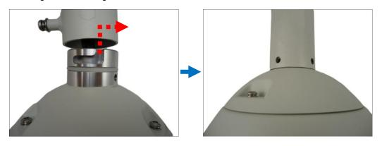
2. Attach the screws included in the camera package to secure the camera.
