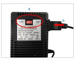
c. Connect the power connector of the camera to the cable connector of the adapter.
