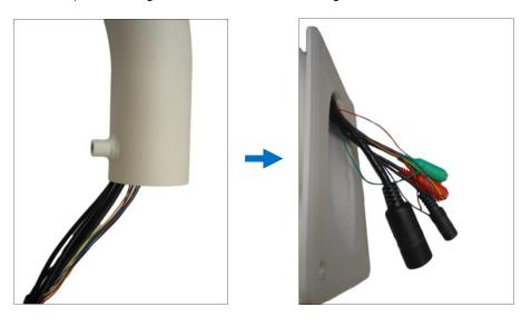
**CAUTION:** The camera itself is waterproof, however take note that the cable connections are not. If the cable connections will be exposed outdoors, make sure to shield or adapt proper waterproofing methods. See *Step 3: Waterproof the Cable Connections* on page 18.
