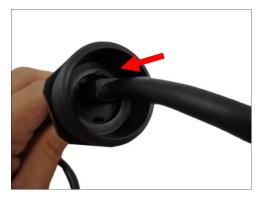
8. Insert the sealing rubber into the conduit gland body.
