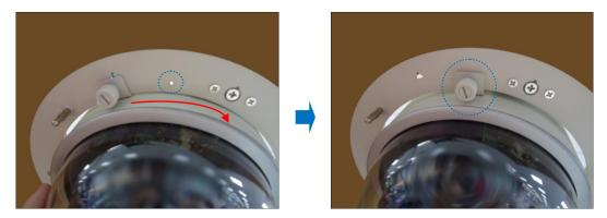
3. Tighten the screw on the fixing bracket to fix the camera position. This is to avoid accidental camera movement as the camera performs PTZ functions.
