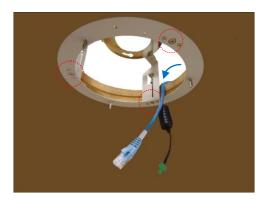
4. Attach the fixing bracket to one of the holes on the camera using the supplied screw (holes marked below). The fixing bracket will fix the camera position when mounted later.
