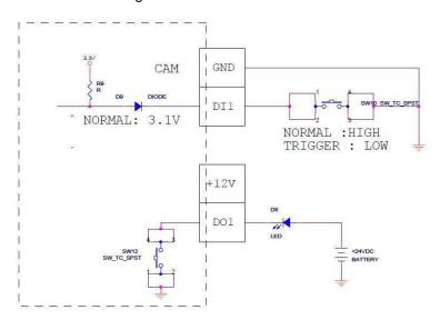
Consequently, to connect a second DI or DO device, use the GND and DI2 pins to connect a second DI device, and the 12V and DO2 to connect a second DO device.
