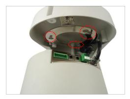
3. Slide the camera clockwise to secure the hooks to the mount.
