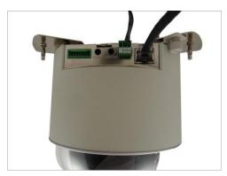
**NOTE:** The cables may be routed along the ceiling if the camera is installed on a hard ceiling. Or, the cables may pass through a hole on the ceiling if the camera is installed on a dropped ceiling.
