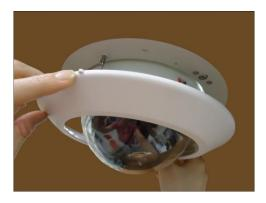
2. Push to firmly secure the cover ring latches.
