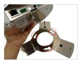
6. Slide the camera clockwise to secure the hooks to the mount.
