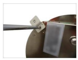
5. Align and insert the camera base hooks to the mounting holes of the metal plate.
