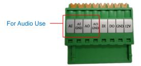
To connect audio devices, map the pins to one of the pin combinations below:
