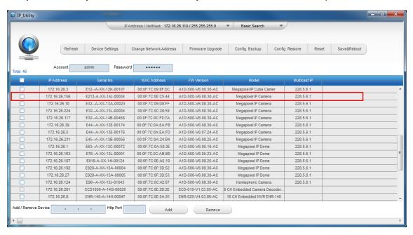
You can quickly notice the camera model in the list. Click on the IP address to automatically launch the default browser of the PC with the IP address of the target camera filled in the address bar of the browser already.
