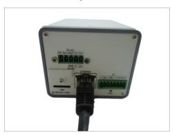
If necessary, connect audio input/output or DI/DO devices to the camera. See How to Connect DI/DO and Audio Devices (Optional) on page 13 for more information.
