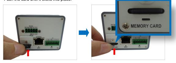
To avoid unauthorize removal of the card, cover the memory card slot. To do this, loosen the screw and turn the tab to cover the memory card slot. Once the tab is in place, tighten the screw.
