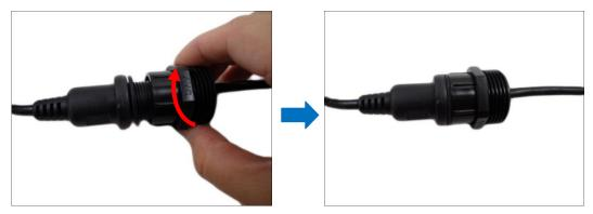
**NOTE:** Make sure the gland body is tightly attached to the "pigtail" and the washer is secured between them.
