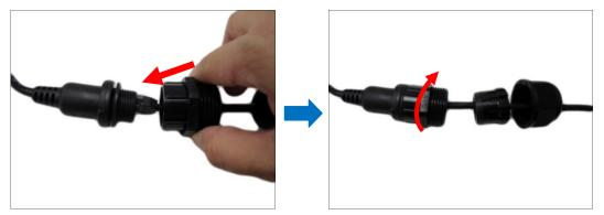
**NOTE:** Make sure the gland body is tightly attached to the "pigtail" and the washer is secured between them.
