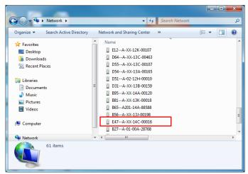
By double-clicking with the left mouse on the camera model, it is possible to automatically launch the default browser of the PC with the IP address of the target camera filled in the address bar of the browser already.
