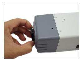
3. Twist and pull to remove the cap covering the threaded end of the lens.
