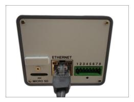
If necessary, connect audio input/output or DI/DO devices to the camera. See How to Connect DI/DO and Audio Devices (Optional) on page 14 for more information.
