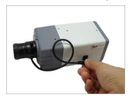
5. Pull to remove the protective cap from the replacement lens.
