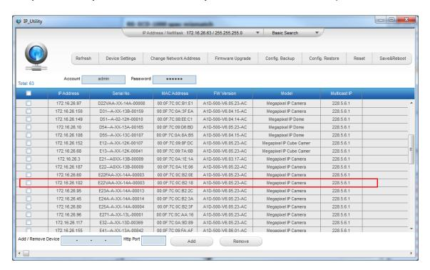
You can quickly notice the camera model in the list. Click on the IP address to automatically launch the default browser of the PC with the IP address of the target camera filled in the address bar of the browser already.
