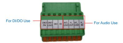
To connect digital input / output devices (DI/DO), map the pins to one of the pin combinations below:
