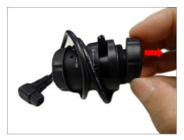
3. Screw the replacement lens to the camera.
