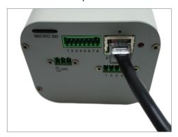
2. If necessary, connect the other external devices, such as DI/DO, PT scanner or power adapter to the camera. See *Before Installation* on page 13 for more information.
