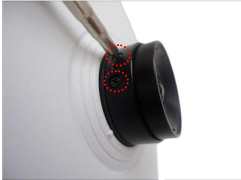
5. Proceed to adjust the camera viewing angle and focus (see [Step 6: Adjust the Viewing Angle and Focus](#) on page 12 for more information).
