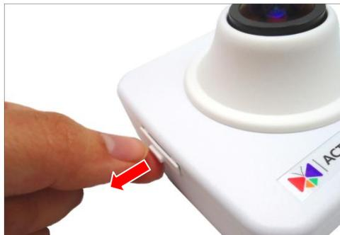
2. Insert the memory card with the metal contacts facing the back of the camera.
