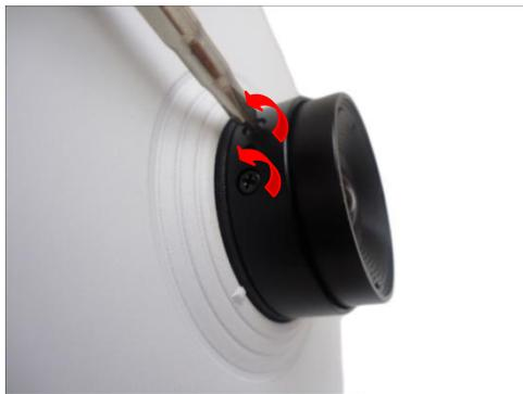
2. Turn the bundled lens counter-clockwise until the lens is detached from its module.
