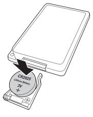
Push the battery compartment back into the slot until it clicks into place.
