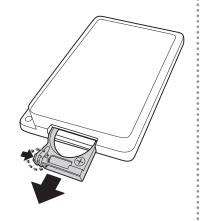
3 Place the battery on the battery compartment.
