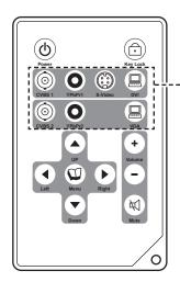
Press the desired input source signal button to select the source.
