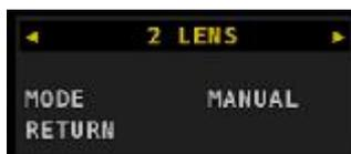
Cameras VCHD-2622, VCHD-4322IR and VCHD-2792IR are equipped with a fix DC-controlled lens. Hence the lens setting has to be set to „DC“.
