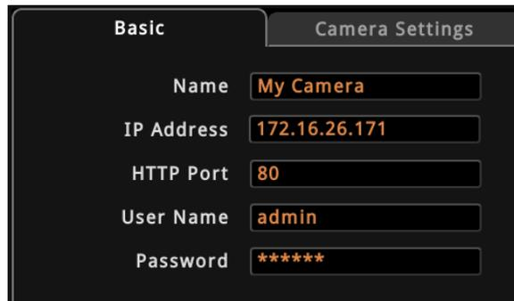
4. Click **Get Camera Settings**. The decoder connects and retrieves the camera settings. At this point, nothing is shown on the Display window yet.
