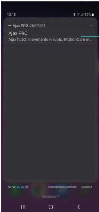
**5** When the **MotionCam** detects a movement it sends, through the Ajax alarm control panel, a notification. Clicking on the notification will open the control screen of the Ajax Pro App
