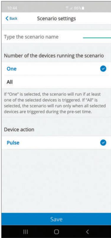
**29** **TYPE THE NAME OF THE SCENARIO** (e.g. Alarm) and select **"ONE"** as device number to activate that scenario
