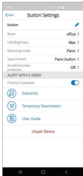
**NOTE:** by activating the PANIC function the ARM-RELAY will remain active leaving the fogging system armed. To restore it, it is needed to manually disarm it from the App or arm and disarm the alarm system.
