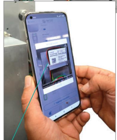
7 Place the camera of your Smartphone in front of the **QR CODE** to acquire, automatically, the ID of the relay device
