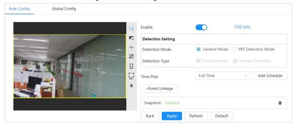
Step 4 Click next to **Enable** to enable the face detection function.
