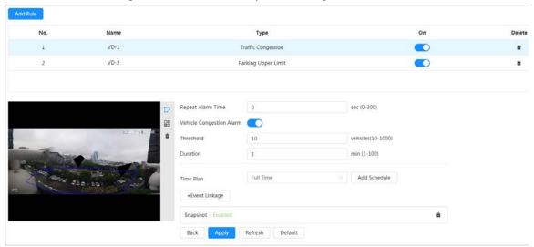
Figure 8-25 Vehicle density (parking upper limit)
