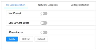
Step 2 Click to enable the SD card detection functions.
