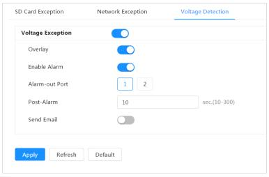
Step 2 Click to enable the voltage detection function.
