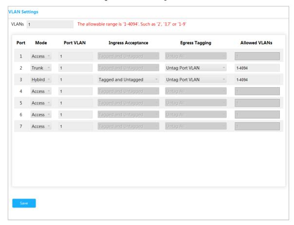
Step 2 Enter 1, 2 in VLANs to create VLAN 1 and VLAN 2.
