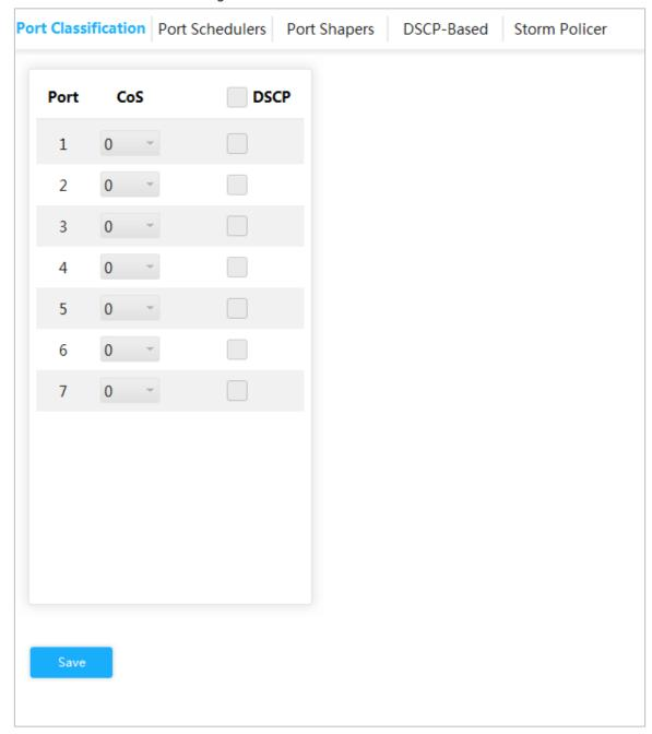
Step 2 Set CoS. For example: Set port 1 to be 1, and port 2 to be 2. See Figure 3-54. Port 1 and port 2 are ingress ports, and port 3 is egress port. The CoS value of port 2 is large than that of port 1, so the data of port 2 will pass port 3 first.
