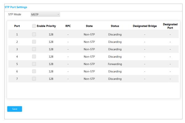
Step 4 Select 3 ports at least to combine an STP/RSTP/MSTP snoop. For example: Port 1, port 2 and port 3 combine an STP snoop. See Figure 3-23.
