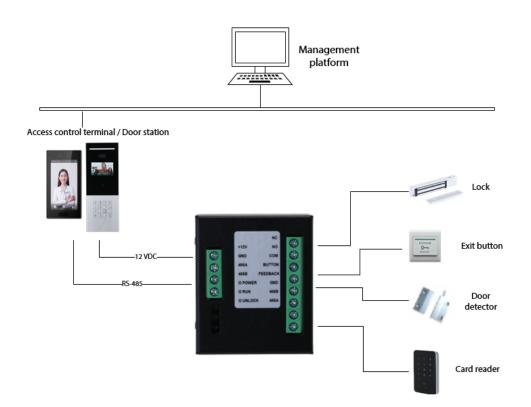
Figure 1-1 Networking diagram
