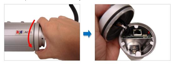
5. To reset the camera, press and hold the Reset button for at least 5 seconds or until the LED lights up.
