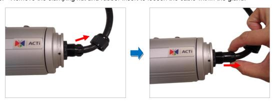
**NOTE:** Connectors are connected inside the camera, be careful when pulling the rubber insert from the gland.
