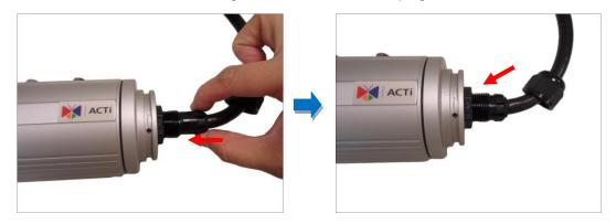
**NOTE:** Make sure the clamping nut is tightly attached to ensure that the connection is waterproof.
