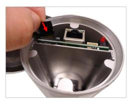
6. Before closing the back cover, make sure the Ethernet cable connector is connected to the main board. If the cable is disconnected, connect as shown below.
