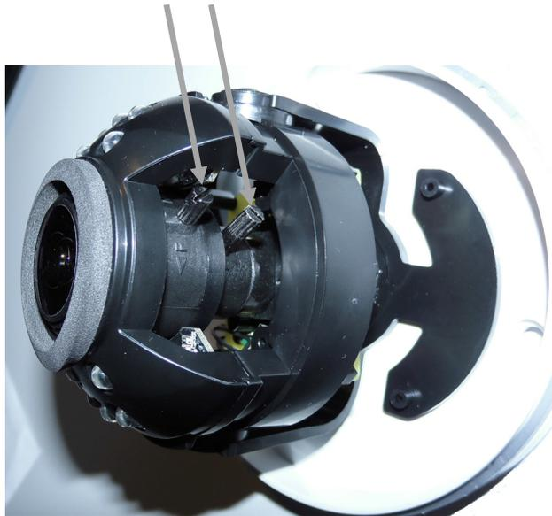
Picture 3: Putting the housing onto the camera module:
