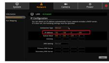
Or, if your network has a DHCP server, select DHCP on Connection Type to obtain an IP address automatically.
